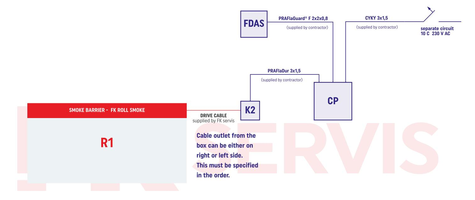
CP: control panel FK ROLL +, 400x300x150 mm, surface mounting, steel box, cable inlet ot top side
