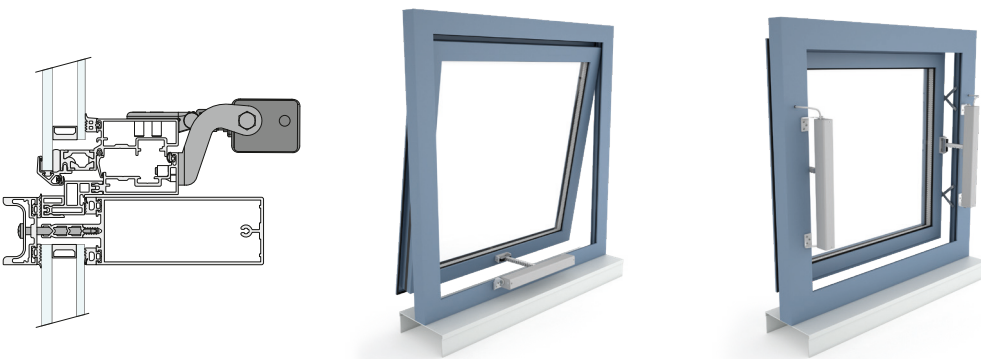
Projected top-hung, parallel opening window, outward opening
